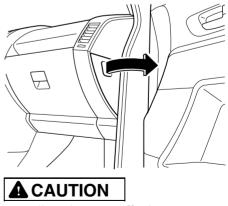
Pulling the cover off sideways may break the retaining tabs off.
